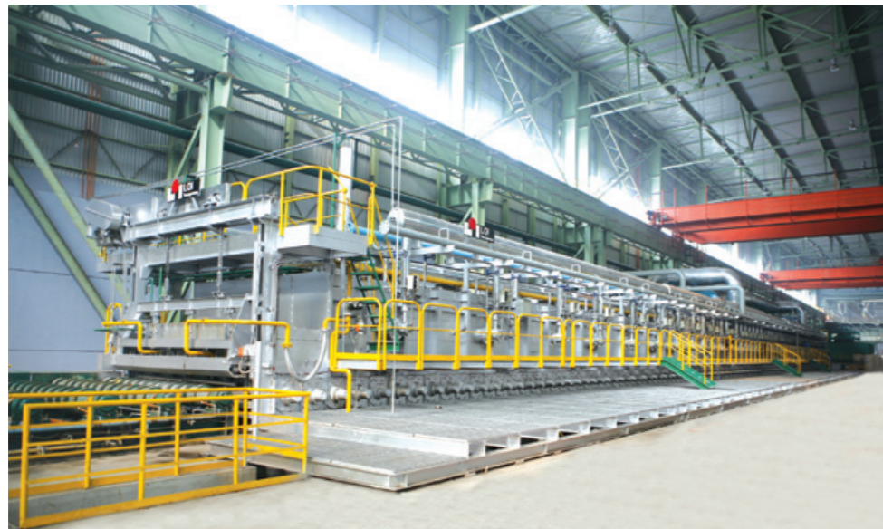
辊底式热处理炉（正火、淬火、回火） Roller type heat treatment furnace (for normalizing, quenching and tempering)
