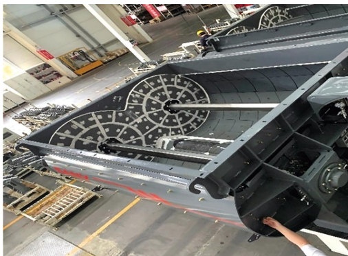
Lining plate in cement mixing tank made of super wear-resistant steel NM450SP
