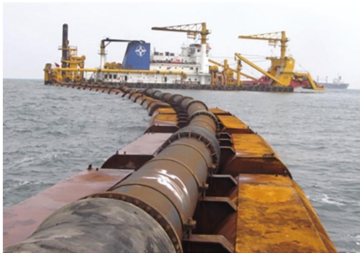
Application of corrosion-resistant and wear-resistant steel in dredged pipes (left) and sanitation trucks (right)
