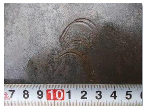
Note to No. 6 Example of flaws remaining on tool of forming device.
