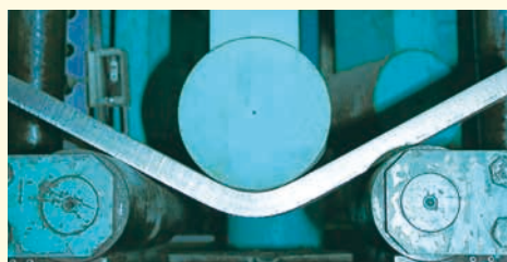
Geometry of bending test piece (JIS Z 2248)
