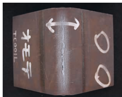
Example of crack which occurred during bending
