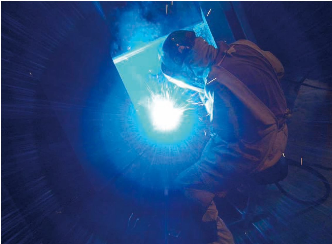
Gas metal arc welding (GMAW): Example of carbon dioxide gas shielded arc welding
