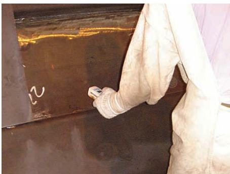
Example of temperature measurement by using a noncontact type thermometer
