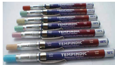
Example of temperature-indicating crayon Temp Stick™, manufactured by Caltech Engineering Services ( http://www.caltechindia.com/TempSticks.htm )
